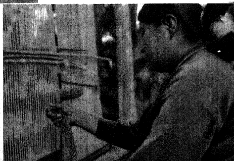
[e] Inserting batten in shed
